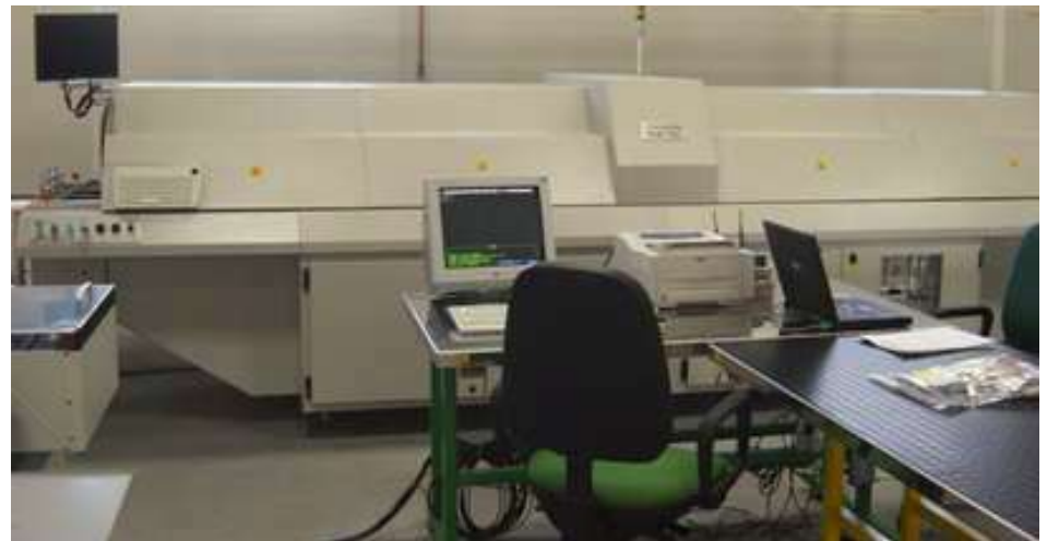
Oven for Soldering Reflow – 14 zones
