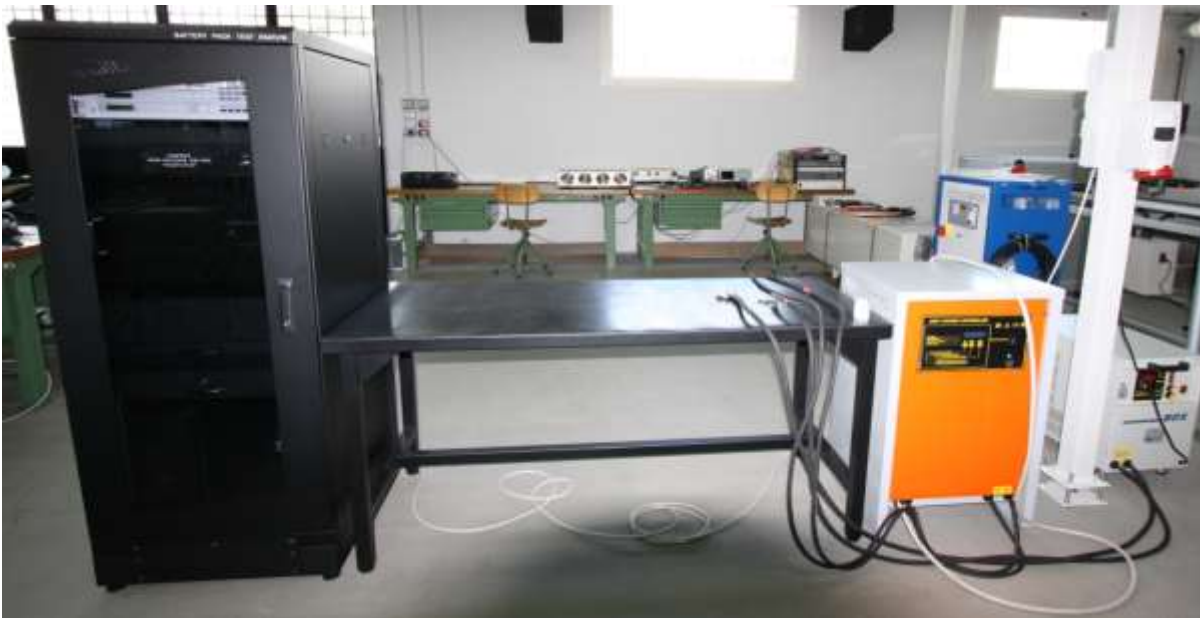
Battery Pack Test Station
